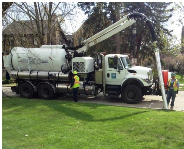
Sewer Division staff operate a sewer cleaning truck to remove debris from a catch basin.
